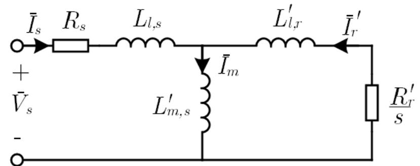
$$\left. \begin{array}{l} \bar{V}_s = R_s \cdot \bar{I}_s + j\omega_s \bar{\Phi}_s \\ 0 = \frac{R_r}{s} \cdot \bar{I}_r + j\omega_s \bar{\Phi}_r \\ \bar{\Phi}_s = L_s \cdot \bar{I}_s + L_m \cdot \bar{I}_r \\ \bar{\Phi}_r = L_r \cdot \bar{I}_r + L_m \cdot \bar{I}_s \\ T_{em} = \frac{3}{2} P_p L_m \operatorname{Im} \left\{ \bar{I}_s \cdot \hat{\bar{I}}_r \right\} \approx \frac{3}{2} \frac{P_p}{R_r} \Phi_s^2 \omega_{slip} \end{array} \right\}$$
